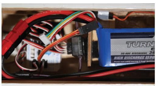
All of these unsecured wires flopping around right over the receiver antenna will cause trouble. There is also 18 inches of wire from the battery to the speed control, and that's WAY too much!
