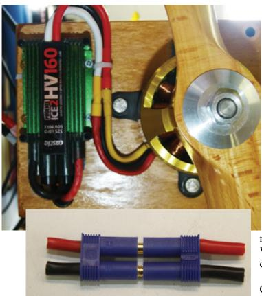
An improper extension made by jamming a bullet into the EC5 connectors. Great connectors ruined by a bad idea.
