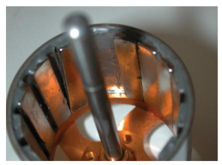
Poorly constructed motors can throw magnets and cause extreme current spikes that will destroy a speed control.
