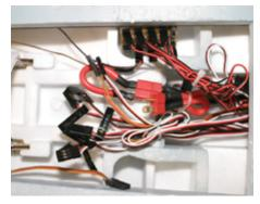
Eleven servos and an onboard LED lighting system overtax the speed control's BEC.
